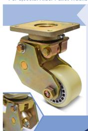
Defining Feature: Designed as a heavier duty quick and easy adjustable from the side of the truck caster. Kingpin-less heavy duty machined & hardened cast housing with no welds and heavy duty 3/8" side plates for added strength and longevity.
