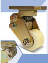
**Defining Feature:** Designed with a full-size swivel mechanism that uses a cup-and-cone with thrust bearing instead of a single-row ball bearing, ensuring high durability and longer wear life.
